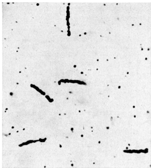
Fig. 12. — The tracks of alpha particles in a boron-loaded plate which had been exposed to a beam of slow neutrons.
